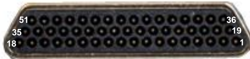
Figure 10 - Pin Location 51-Pin
